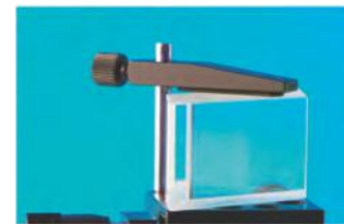
Optics is held by rubber padded clamp
